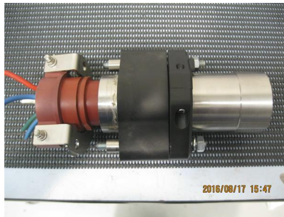
5 Pin BBL socket assembly previously certified to AUSEx 3818U
