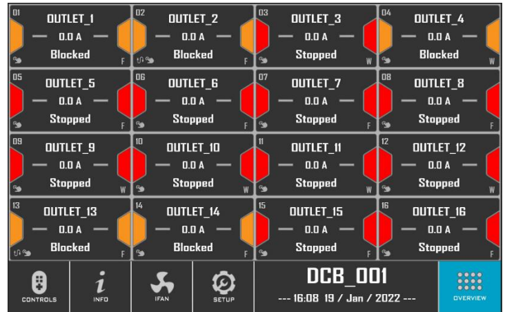
Protection Interface Platform GUI (max of 16 outlets shown)
