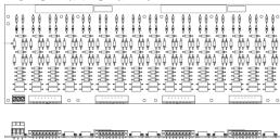
The modules comprise of a printed circuit board upon which are mounted electronic components which provide voltage and current limitation via a triplicated arrangement of shunt voltage limiter circuits and series current limiting resistors respectively. Electrical connections are made either via screw terminal blocks or keyed ribbon cable connectors.
