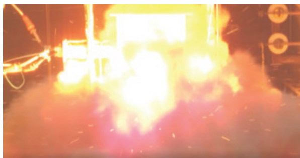
Venting the arc blast may be hazardous in an underground mine
