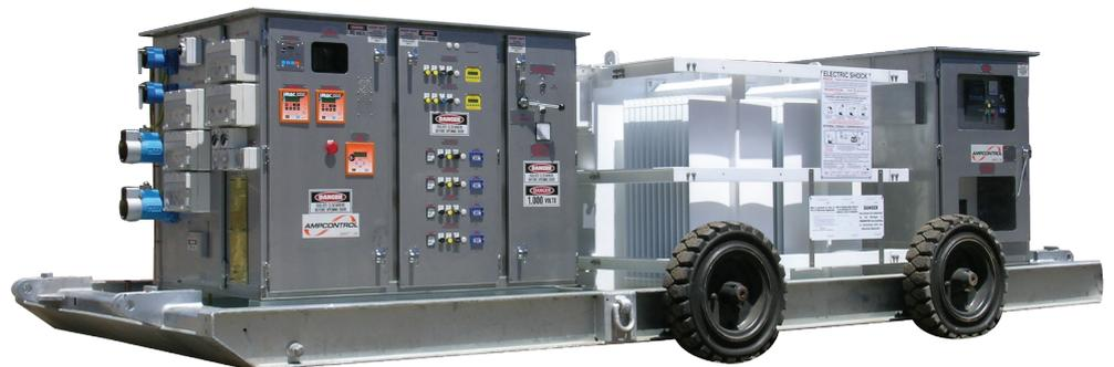
11kV connections are typically provided via a flameproof coupler. All 11kV equipment is housed in the High Tension (HT) Enclosure of the substation. The HT Enclosure may incorporate switched or non-switched through supplies and 11kV DOL Conveyor Motor Starters. Integrated into the HT enclosure are the isolation, earthing and protection required for the main transformer. Protection will include meeting all requirements for electrical protection of a substation as detailed in AS4871.2012.
